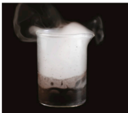
FIGURE 18.3.7 The decomposition of hydrogen peroxide is usually very slow, but the addition of crystals of potassium permanganate results in the rapid evolution of oxygen gas and water vapour.
