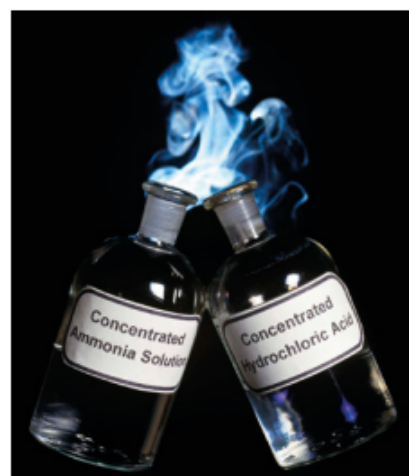
FIGURE 14.1.7 White ammonium chloride powder is formed as gases from concentrated ammonia solution and hydrochloric acid solution diffuse from their containers and react. Ammonia and hydrogen chloride are colourless gases.
