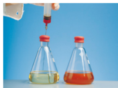
FIGURE 8.4.10 Test for unsaturation. Adding a few drops of orange-coloured bromine solution to hexane (right) produces no immediate reaction. In sunflower oil (left), the colour of the bromine solution disappears almost immediately because molecules in the sunflower oil contain carbon-carbon double bonds, which undergo addition reactions with bromine (Br 2 ).
