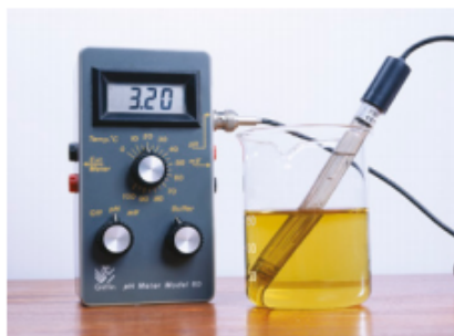
FIGURE 17.2.7 A pH meter is used to measure the acidity of a solution.
