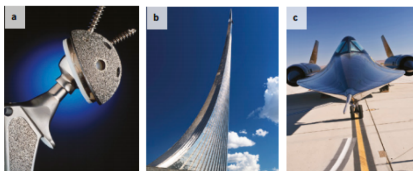
FIGURE 4.1.1 Titanium has many uses: (a) a replacement hip socket, (b) the spectacular curved space museum building in Moscow and (c) the SR-71 Blackbird reconnaissance aircraft. The SR-71 aircraft was the fastest piloted aircraft that used oxygen directly from the atmosphere.
