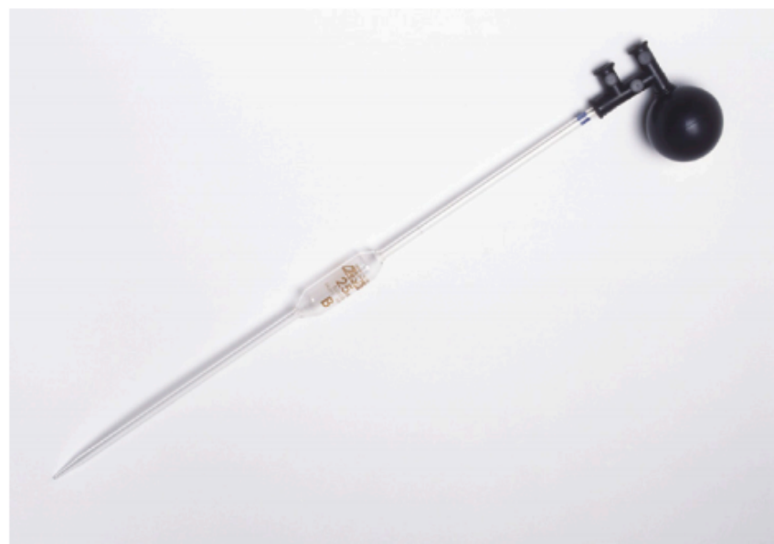
FIGURE 20.3.1 Record the uncertainty for glassware and instruments. This pipette can dispense a volume (aliquot) of 25.00 \pm 0.03 mL. When used correctly, the volume dispensed will be between 24.97 mL and 25.03 mL.
