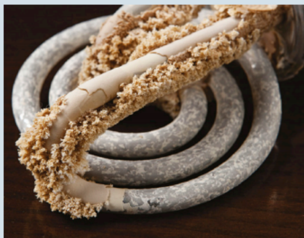
FIGURE 16.1.5 The accumulation of limescale on domestic kettles is the result of precipitation of calcium carbonate as water is repeatedly boiled.
