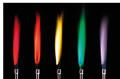
FIGURE 3.5.2 The colour of a flame is different in the presence of different metal compounds and can be used to identify the presence of these metals. The flame colours shown here indicate the presence of (left to right) lithium (red), strontium (red), sodium (yellow), copper (green) and potassium (lilac).
