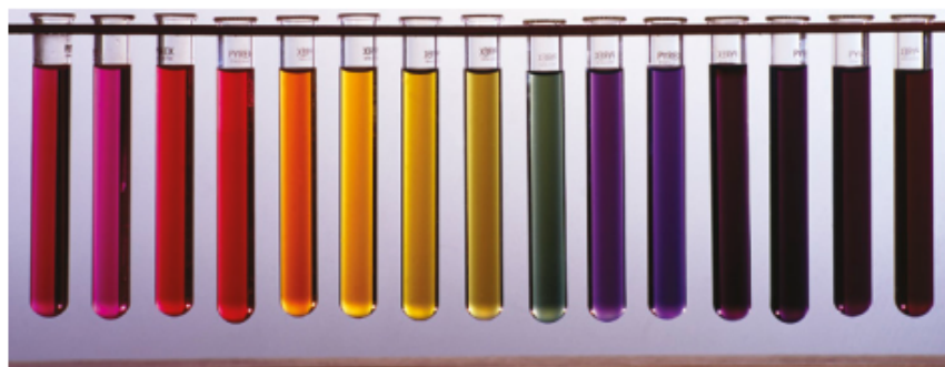
FIGURE 17.1.2 Universal indicator pH scale. When universal indicator is added to a solution, it changes colour depending on the solution's pH. The tubes contain solutions of pH 0 to 14 from left to right. The green tube (centre) is neutral, pH 7.
