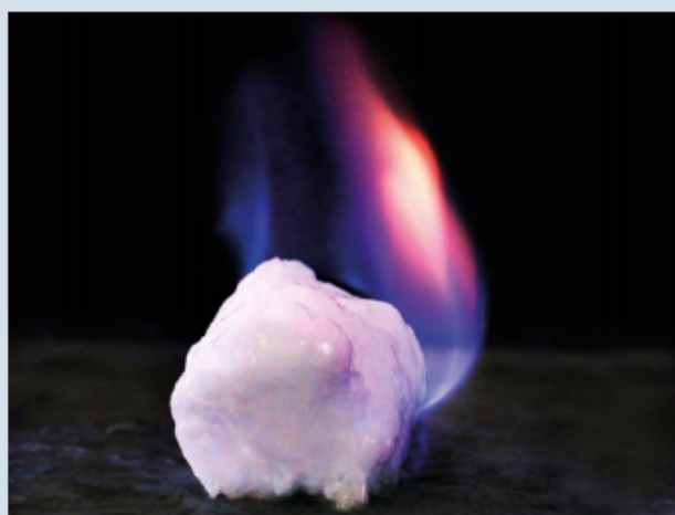
FIGURE 8.1.9 The combustion of blocks of methane hydrate gives the appearance of burning ice. As the ice melts, methane gas is released from the lattice structure, providing the fuel for the combustion reaction.
