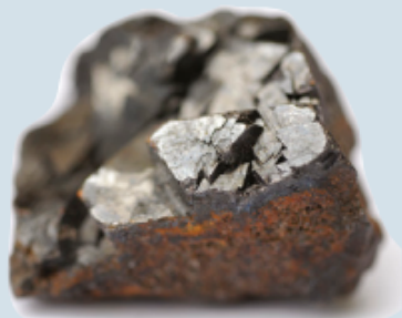
FIGURE 9.4.3 Elemental analysis of the mineral magnetite has allowed chemists to determine the percentage composition to be 72.4% iron and 27.6% oxygen.
