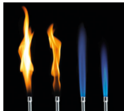
FIGURE 11.2.1 The yellow flame of a Bunsen burner is due to incomplete combustion and produces carbon as a product. The blue flame is a hotter flame that occurs when the collar hole is open and more oxygen is allowed into the reaction. Complete combustion can then occur.
