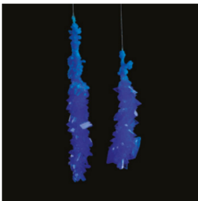
FIGURE 15.6.6 Large crystals of copper(II) sulfate formed by slowly cooling a saturated solution of the compound
