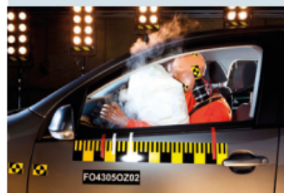
FIGURE 14.1.4 An airbag deploys in a test car within 30 milliseconds of impact, with a crash dummy taking the impact.
