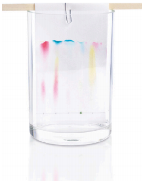
FIGURE 13.1.5 Paper chromatography can be used to separate mixtures of inks into their separate components.
