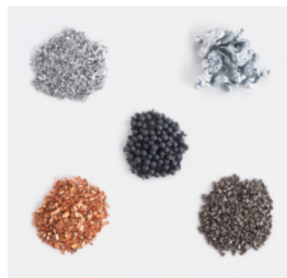
FIGURE 1.1.1 An example of different metals (clockwise from the bottom left): copper, aluminium, zinc, iron and, in the centre, lead
