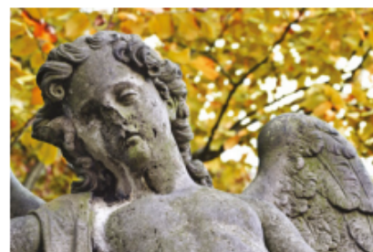
FIGURE 17.3.4 This statue has been heavily eroded by acid rain, which reacts with carbonate salts in limestone. Acid rain is formed when gases, such as sulfur dioxide and nitrogen oxides, dissolve in water to form acidic solutions.
