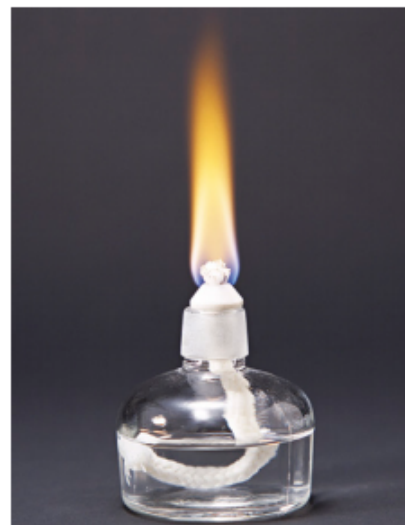
FIGURE 11.3.1 Ethanol burning in a spirit burner. Combustion of 1 gram of ethanol releases almost 30 kJ of energy.
