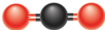
FIGURE 12.1.9 In a carbon dioxide molecule, the carbon atom forms double bonds with two oxygen atoms. The two double bonds repel each other. This results in a linear molecule.
