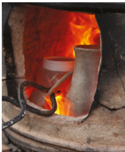
FIGURE 5.2.1 Bricks made from the ionic compound magnesium oxide are used to line furnaces and kilns.
