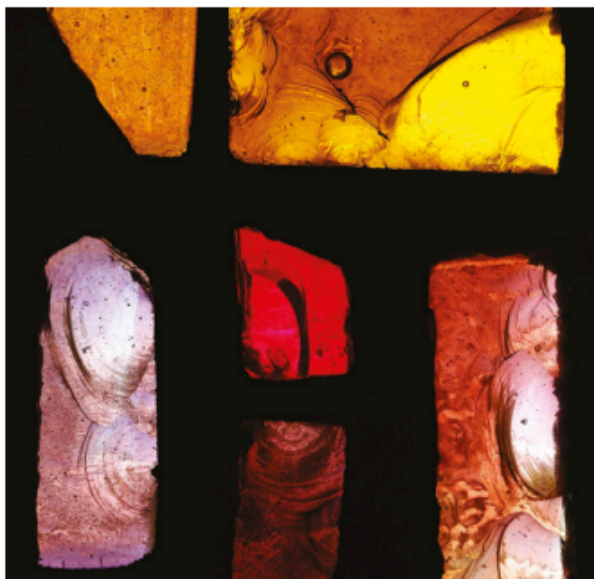
FIGURE 1.2.7 The red colour in this stained glass window is caused by gold nanoparticles trapped in the glass. The deep yellow colour is caused by silver nanoparticles.
