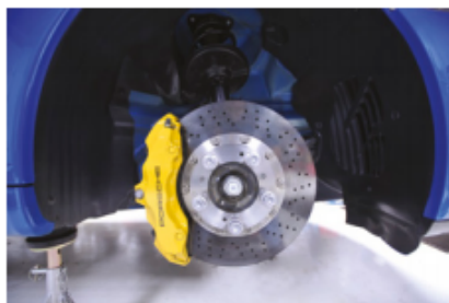
FIGURE 5.2.2 Ceramic brake discs work more effectively than steel ones at high temperatures. A ceramic brake disc contains ionic compounds that have very high melting temperatures and withstand the heat produced by braking better than metals.
