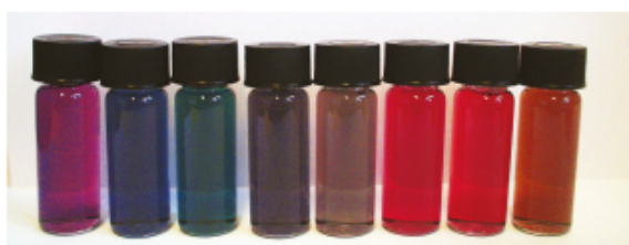
FIGURE 1.2.6 These vials contain gold particles of various sizes. The different-sized particles are different colours because they interact with light differently.
