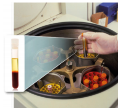
FIGURE 1.3.7 Centrifuges like this one are used to separate the components of blood in small quantities. Blood that has been centrifuged separates into three distinct layers. The top layer is the plasma, the middle layer is the buffy coat and the bottom layer is composed of red blood cells.
