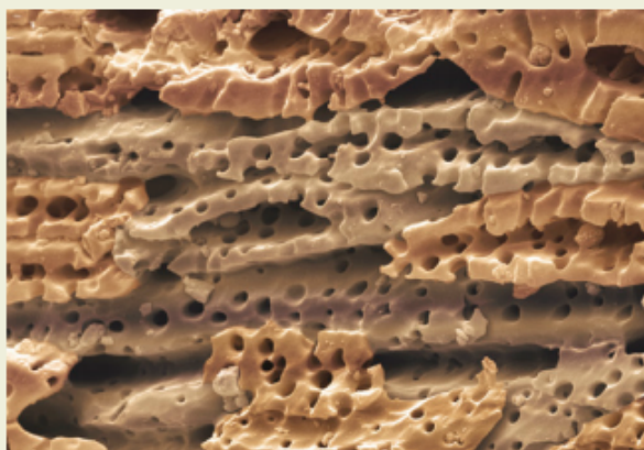
FIGURE 7.1.17 A microscope image of activated charcoal shows that it contains many pores and hollows.
