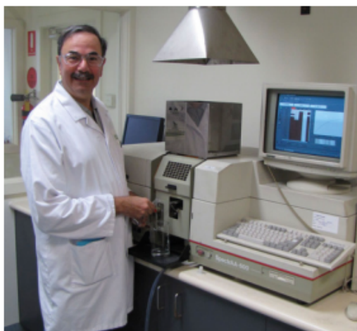
FIGURE 3.5.3 An analytical chemist uses AAS to determine the concentration of metals in food.
