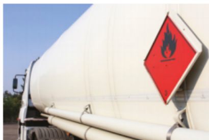
FIGURE 20.2.7 Trucks transporting hazardous substances, such as flammable liquids, have hazard symbols attached.
