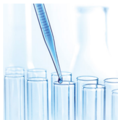
FIGURE 20.2.3 A 5 mL graduated pipette can measure volumes to an accuracy of one hundredth of a millilitre, or 5 \text{ mL} \pm 0.01 \text{ mL} . The pipette has major divisions of 1 mL and minor divisions of 0.1 mL. You can estimate to 0.01 mL and record volumes to 2 decimal places, for example 3.80 mL or 4.52 mL.
