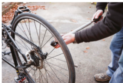
FIGURE 14.1.9 Pumping more air into a tyre increases the pressure in the tyre because more particles are being pumped into a nearly fixed volume.
