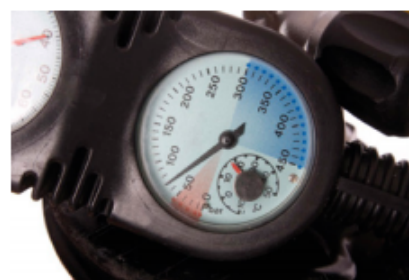
FIGURE 14.1.11 A pressure gauge like this one would be found on a cylinder of compressed air used in scuba diving.
