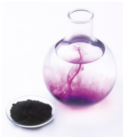
FIGURE 15.3.1 When solid potassium permanganate is added to water, it dissolves. The particles disperse into the solution and move around freely.
