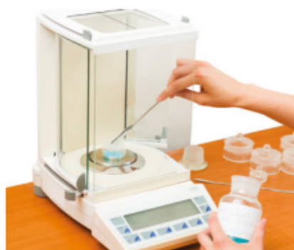
FIGURE 9.3.1 A digital balance is a piece of laboratory equipment used for weighing.
