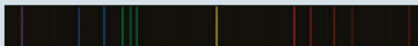
3.4.11 The emission spectrum of helium is made up of lines ranging from violet to red in colour.
