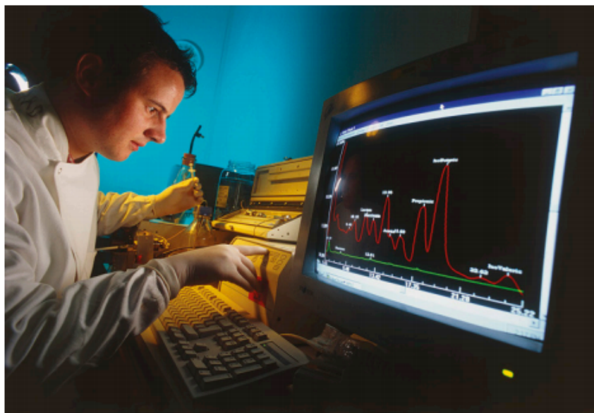
FIGURE 13.2.3 A research chemist using high-performance liquid chromatography to analyse the components in a mixture for medical research
